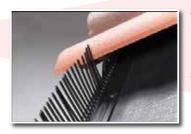
The Eaves Comb Filler (Bird Comb) creates a barrier against birds and large insects. It prevents them entering the void between the underside of Profiled Tiles and the underlay on pitched roofs. Injection moulded from high quality, low density polyethylene. It's flexibility prevents any alignment problems. Manufactured in 1.0mtr strips, which is effective, quick and easy to fit. Durable and totally resistant to decay.
