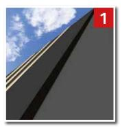
1. Install the underlay and battens as normal, leaving the underlay 5-30mm short of the ridge on both sides. Do not fix the top tiling batten at this stage.
