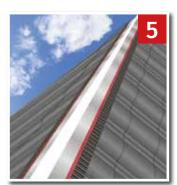
5. Roll out the ridge roll centrally across the entire length of the ridge batten, using the white spine of the roll as a guide over the ridge batten. Secure the roll by nailing or stapling through the white spine. All joints must be overlapped by 75mm min. Leave a 75mm long strip of the roll at each end of the ridge.
