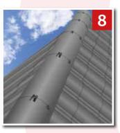
8. Continue this process along the ridge to the end. Secure the ridge end tile through the pre-drilled holes provided, or drill a hole through when using a reclaimed tile.
