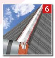
6. Remove the release paper from the butyl adhesive strip on the underside of each edge of the ridge roll, and firmly press onto the clean dry tile on both side, avoid crushing the corrugations. Continue this process along the entire ridge line. Adhere the roll to the vertical surface of the dry verge at the gable end and at the hip abutment, overlap the roll across the hip rolls by 75mm, carefully sealing the butyl adhesive in place.
